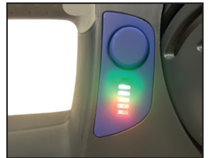
❻. The battery indicator will illuminate from Red (Low battery) ---Amber---Green (fully charged). The lights will turn off once fully charged.
